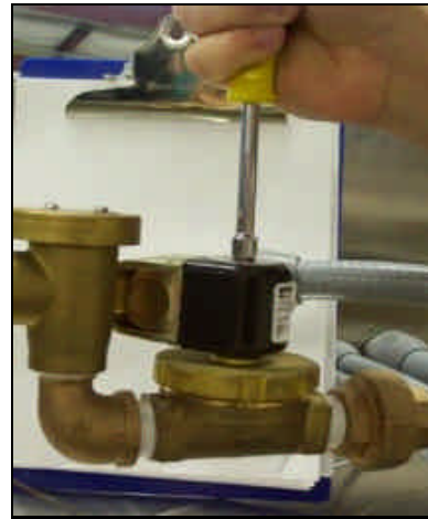
Removing the top screw
